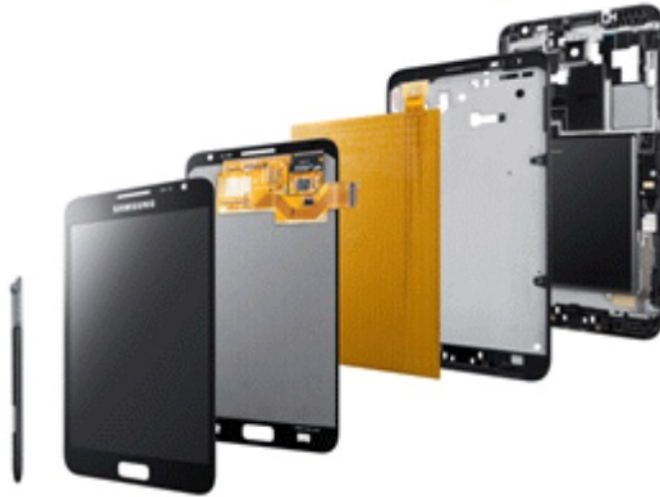
Fig. 1 Configuration of electromagnetic induction type electronic pen input device
