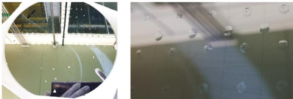
Figure 6. Fabricated wafer-scale lens after CMP process
