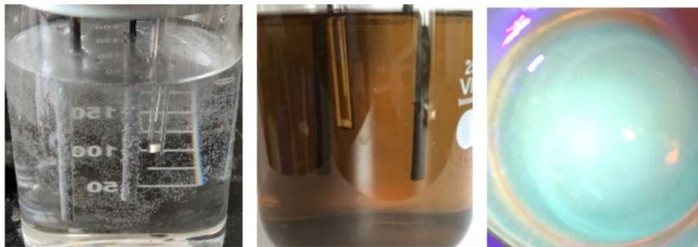
Fig. 2.1. Variation diagram of the reaction process of carbon quantum dots prepared by electrochemical
