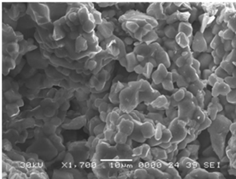
Fig. 2: Scanning electron microscopy image of the synthesized  $\text{NaBaY}_{0.5}(\text{MoO}_4)_3:\text{Eu}_{0.05}\text{Yb}_{0.45}$  particles.
