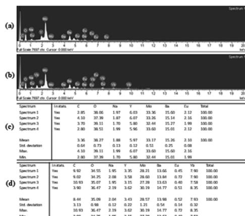
Fig. 3: Energy-dispersive X-ray spectroscopy patterns of the synthesized (a)  $\text{NaBaY}_{0.8}(\text{MoO}_4)_2:\text{Eu}_{0.2}$  and (b)  $\text{NaBaY}_{0.5}(\text{MoO}_4)_2:\text{Eu}_{0.05}\text{Yb}_{0.45}$  particles, and quantitative compositions of (c)  $\text{NaBaY}_{0.8}(\text{MoO}_4)_2:\text{Eu}_{0.2}$  and (d)  $\text{NaBaY}_{0.5}(\text{MoO}_4)_2:\text{Eu}_{0.05}\text{Yb}_{0.45}$  particles.
