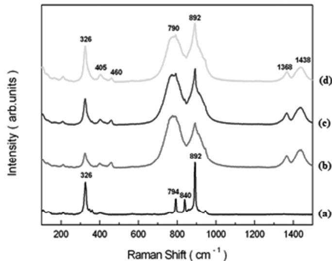
Fig. 5: Raman spectra of the synthesized (a)  $\text{NaBaY}(\text{MoO}_4)_3$ , (b)  $\text{NaBaY}_{0.8}(\text{MoO}_4)_3:\text{Eu}_{0.2}$ , (c)  $\text{NaBaY}_{0.7}(\text{MoO}_4)_3:\text{Eu}_{0.1}\text{Yb}_{0.2}$ , and (d)  $\text{NaBaY}_{0.5}(\text{MoO}_4)_3:\text{Eu}_{0.05}\text{Yb}_{0.45}$  particles excited by the 514.5-nm line of an Ar ion laser at 0.5 mW.
