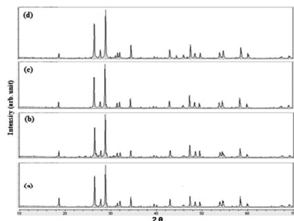
Fig. 1: X-ray diffraction patterns of the synthesized (a)  $\text{NaBaY}(\text{MoO}_4)_3$ , (b)  $\text{NaBaY}_{0.8}(\text{MoO}_4)_3:\text{Eu}_{0.2}$ , (c)  $\text{NaBaY}_{0.7}(\text{MoO}_4)_3:\text{Eu}_{0.1}\text{Yb}_{0.2}$  and (d)  $\text{NaBaY}_{0.5}(\text{MoO}_4)_3:\text{Eu}_{0.05}\text{Yb}_{0.45}$  particles.
