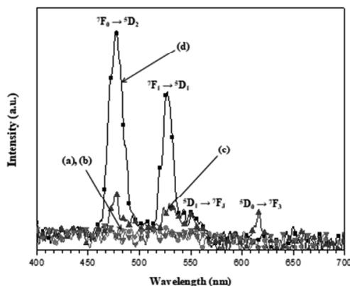
Fig. 4: Upconversion photoluminescence emission spectra of (a)  $\text{NaBaY}(\text{MoO}_4)_3$ , (b)  $\text{NaBaY}_{0.8}(\text{MoO}_4)_3:\text{Eu}_{0.2}$ , (c)  $\text{NaBaY}_{0.7}(\text{MoO}_4)_3:\text{Eu}_{0.1}\text{Yb}_{0.2}$  and (d)  $\text{NaBaY}_{0.5}(\text{MoO}_4)_3:\text{Eu}_{0.05}\text{Yb}_{0.45}$  particles excited under 980 nm at room temperature.
